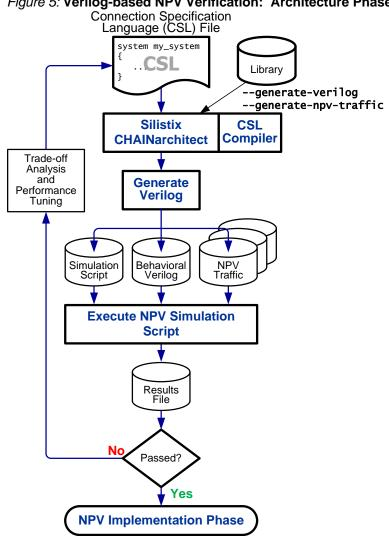
Figure 5: Verilog-based NPV Verification: Architecture Phase
