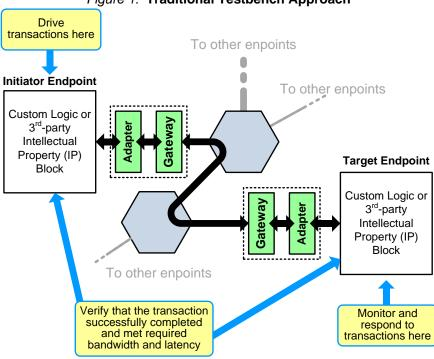
Figure 1: Traditional Testbench Approach
