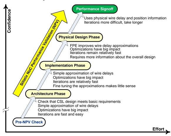
Figure 3: Silistix NPV Performance Closure Process
