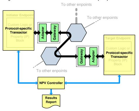
Figure 2: Automated NoC Performance Validation (NPV) Environment
