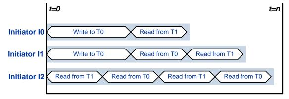
Figure 16: Three Initiator Blocks within a Mode
